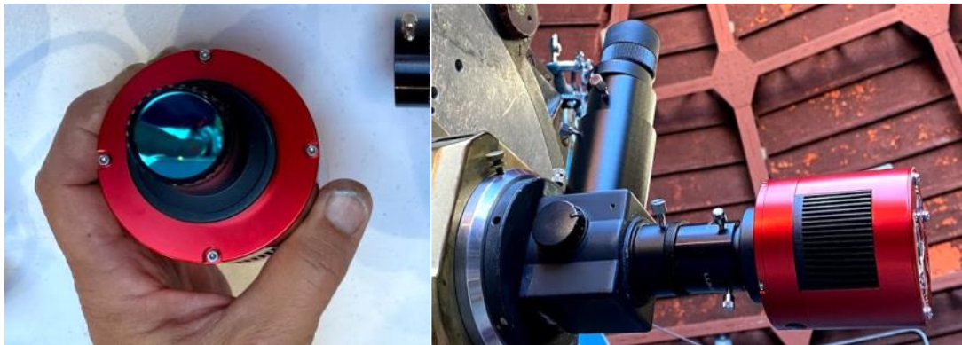
Figure 2: (Left) Red filter on the ZWO camera; (Right) ZWO ASI 1600 Camera attached to a flip mirror with an eyepiece at the top.
