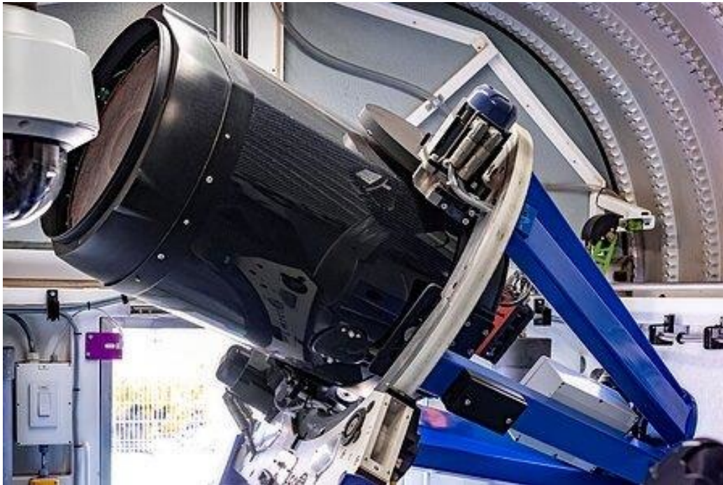
Figure 3. Las Cumbres Observatory 0.4-meter Telescope Faulkes Telescope North Haleakalā Observatory. Telescope style: Cassegrain reflector optical telescope, Ritchey-Chretien telescope atop Haleakala (3,055m) Maui County. Hawaii, USA.
