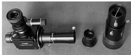
Figure 1. From left to right: flip mirror with 5x Powermate, nose piece with 0,5X reducer field lens, ocular projection unit with Plössl eyepiece and suspended occulter and camera. Overall focus is adjusted using the camera distance from the transfer eyepiece.
