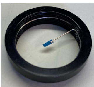
Figure 6. Improved method for carrying a 'free standing' occulter. Here, it is mounted on a separate filter ring but the method is easily transferable to the internal thread of the transfer eyepiece itself.
