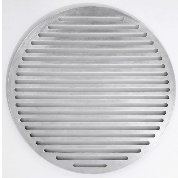
Figure 1: Aluminum diffraction grating used to establish the image scale
