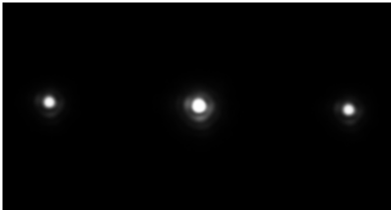
Figure 2: H-alpha diffraction image of Capella through the 254-mm refractor
