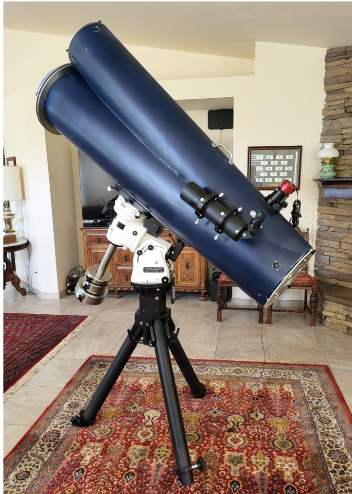
Figure 2: Completed tube assembly of 310-mm f/15 folded refractor on AP-1100 mounting
