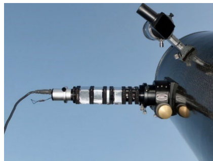
Figure 1 : High Contrast Double Star Filter (HCDSF) instrument mounted on ocular adapter on the 12-inch Newtonian telescope
