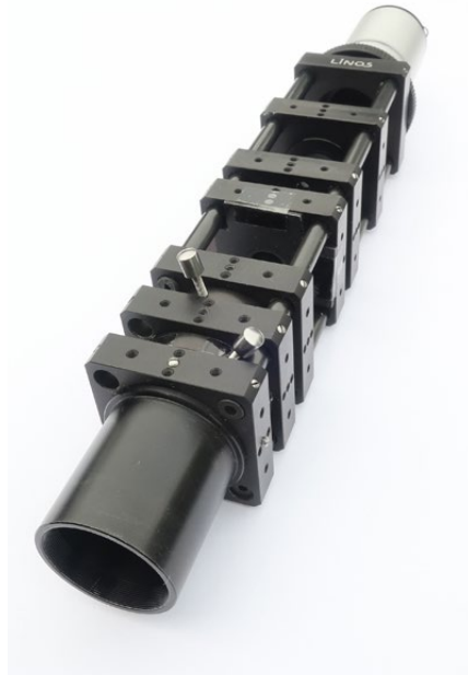
Figure 1 : High Contrast Double Star Filter (HCDSF) instrument, ocular sleeve and filter unit in foreground, optical unit and CMOS camera in background. The filter unit consist of a polarization foil F1 and a polarization stripe F2.
