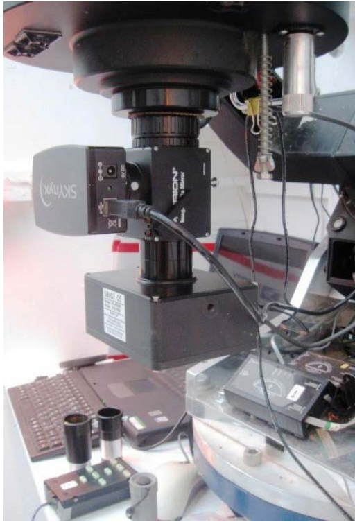
Figure 2: Instrument cluster on the back of the 10-inch telescope. An Orion Telescopes flip mirror is directly below the telescope, with the Luminera high speed camera to the left of the flip mirror and the SBIG ST-402 camera below it.
