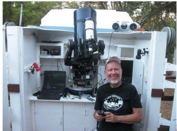
Figure 1: The author and 10-inch telescope at the Orion Observatory. The laptop on the left controls the telescope and acquisition camera, while the laptop on the right controls the high-speed Luminera camera.
