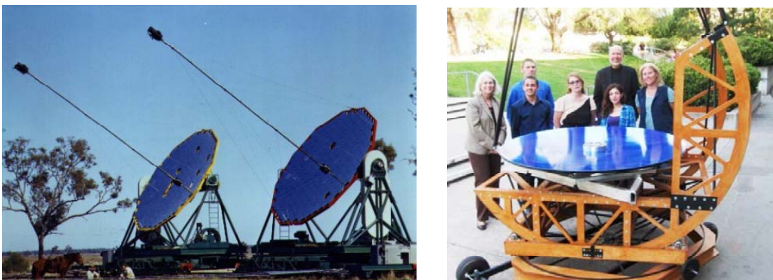
Figure 14: Hanbury Brown's stellar intensity interferometer in Narrabri, Australia (left). On the right is the portable 1.5 meter light bucket telescope designed and built by Russ Genet and students at California Polytechnic State University.
