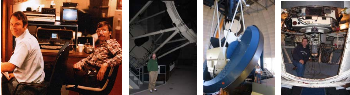
Figure 20: Bill's early speckle career included runs at the 4-meter telescope at Kitt Peak National Observatory. Data was logged on an early Osborne microcomputer. The speckle interferometry camera was installed at the Cassegrain focus. That's Bill in the "Cass cage."
