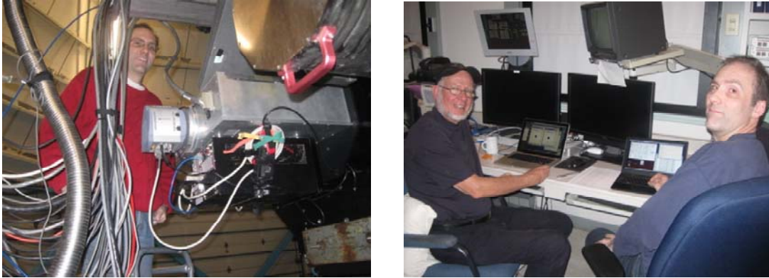
Figure 11: Elliott Horch and his two-channel speckle interferometer mounted on one of the two Nasmyth foci of the 3.5 meter WIYN telescope at Kitt Peak. One of the two Andor iXon EMCCD cameras can be seen as well as a PC strapped to the bottom of the photometer. Russ and Elliott in the warm room during a recent run.
